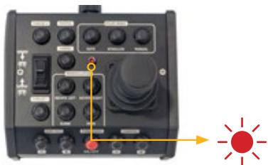
The Oceanus hand controller is equipped with a power indicator light. The light will glow brightly indicating the hand controller is properly connected in an USB port found in the topside and is receiving power. Your hand controller may be furnished with either a red or green indicator light.
