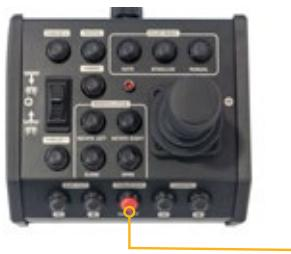
As a safety precaution the power relay to thrusters is set to an “Off” position, meaning the thrusters are inoperable. Push the Thruster Off/On button once to set the power relay to thrusters to the “On” position. Thrusters will respond to corresponding thruster commands.
